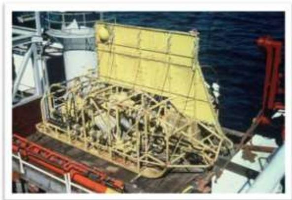
*Figure 8: Two-metre DOMCO hydraulic collector*
