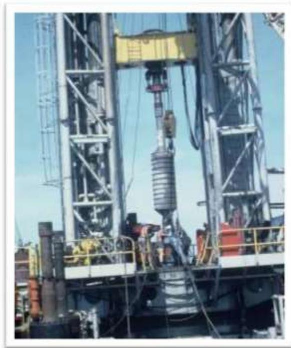
*Figure 11: Deadweight being installed*
