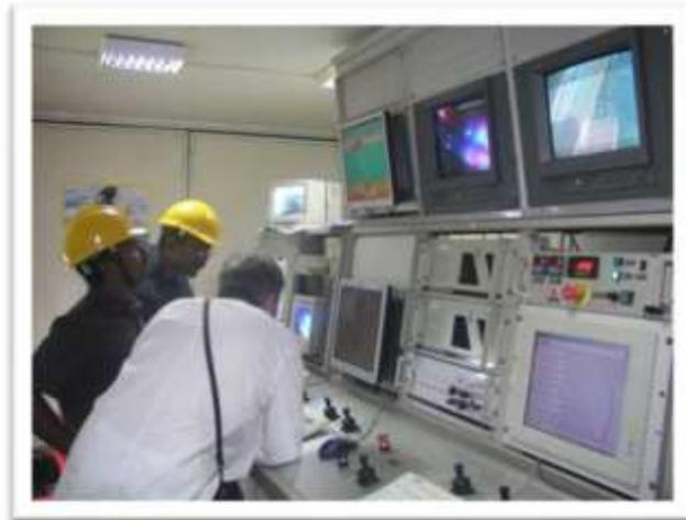
*Figure 11: Control panel for in-situ soil tester*
