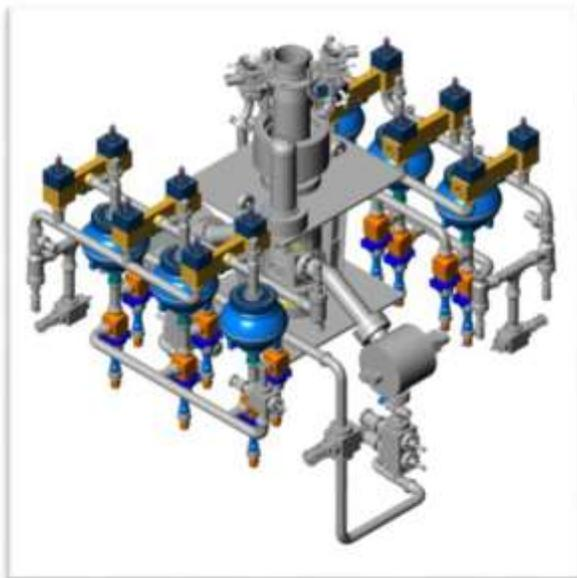
*Figure 18: Subsea mud pump (Hydril)*
