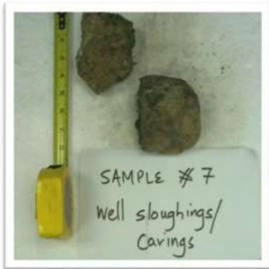
*Figure 20: Solids pumped through the SMP*
