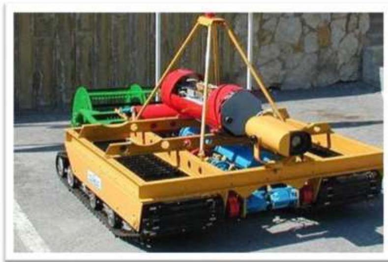
*Figure 5: Model of self-propelled collector*
