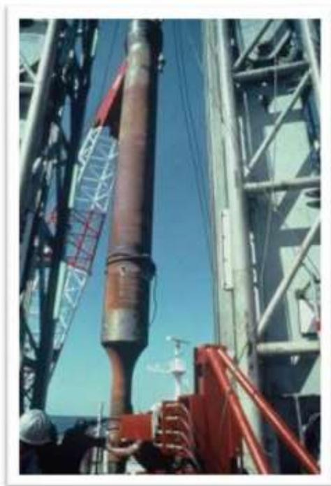
*Figure 12: In-line submersible pump*
