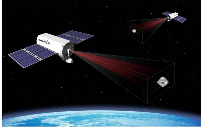
**Figure 1 XSS-11 spacecraft equipped with the MDA Space borne Scanning Lidar System**
