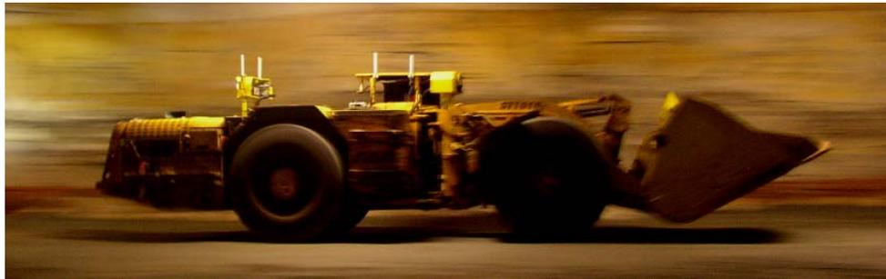
**Figure 2 Underground Load Haul Dump (LHD) vehicle driving autonomously with no infrastructure (right)**
