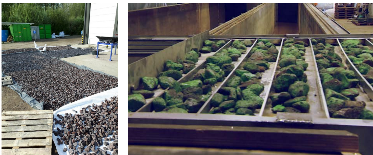
Figure 121: Lava stones handling : Lava stones being separated into different sizes (left) and 1 m 2 of nodule traveling carriage (right)
