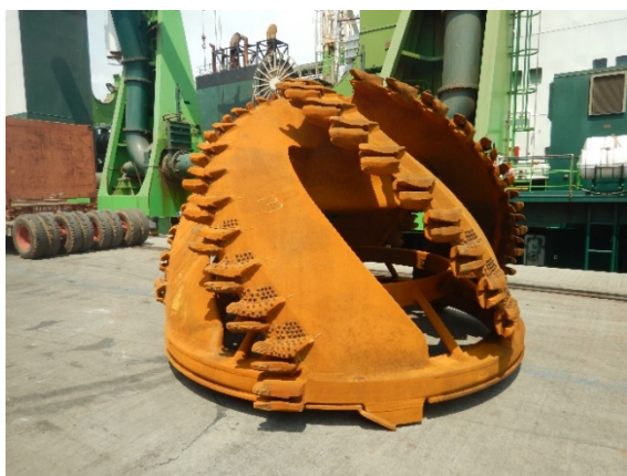
Figure 113: Analogy with cutter heads allowing geometrical variations depending on the soil : Sand cutter head on CSD Ambiorix– open design (left) and Rock cutter head on CSD Ambiorix – robust and “closed” design (right)
