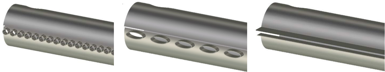
Figure 115: Geometrical configurations (CFD Part 1) : (1) Circular configuration (left), (2) Ellipsoid configuration (centre) and (3) Rectangular configuration (right)
