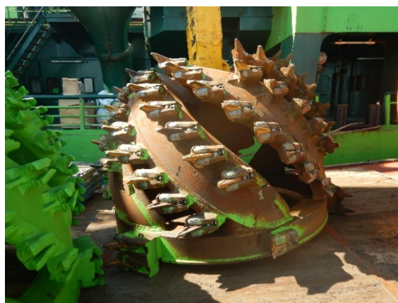
Figure 113: Analogy with cutter heads allowing geometrical variations depending on the soil : Sand cutter head on CSD Ambiorix– open design (left) and Rock cutter head on CSD Ambiorix – robust and “closed” design (right)
