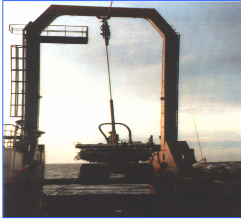
Figure 12: Launching of underwater mining system.
