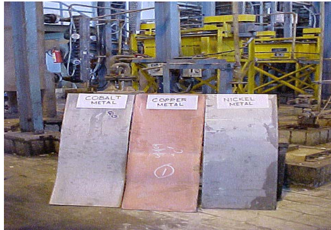
Figure 21: Cathode Sheets from Pilot Plant.
