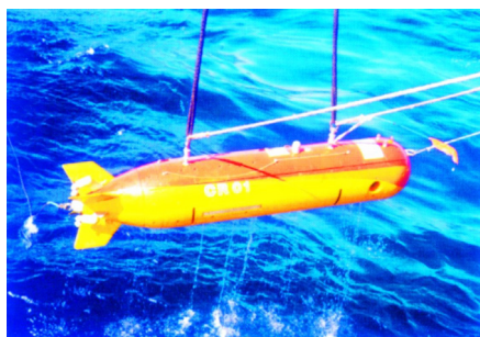
Figure 4: Deep seabed exploration technology development –Autonomous underwater vehicle.
