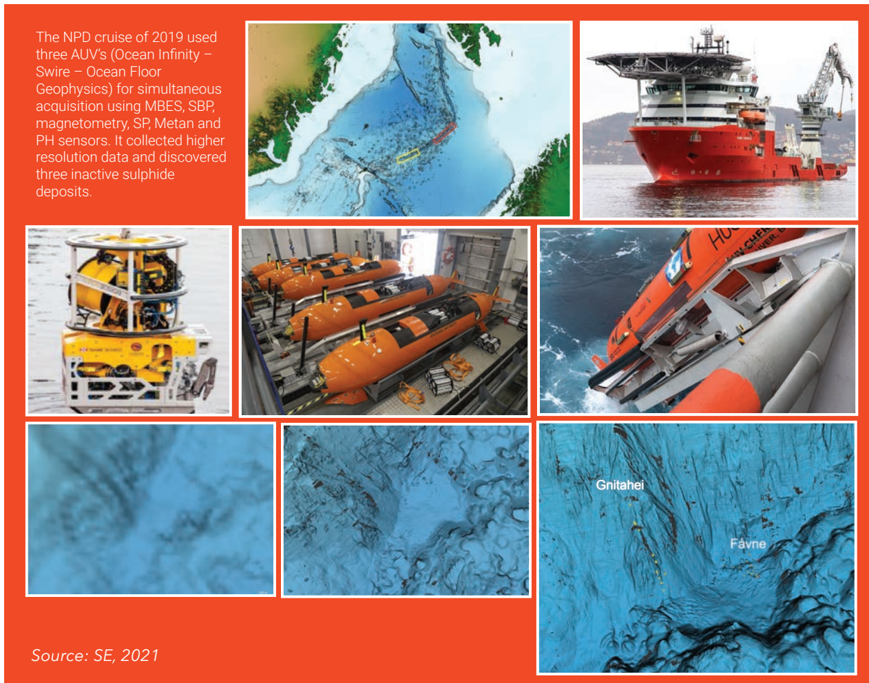
Figure 8. Use of AUVs during the NPD cruise in 2019
