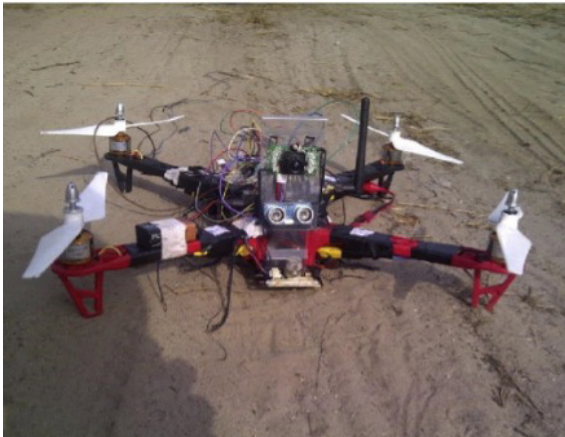
Figure 12. Drone used for collection of aerial (weather) data
