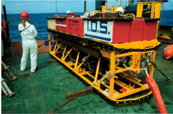
Figure 10: The Southampton Oceanography Centre's deep-tow sidescan sonar instrument TOBI being prepared for launch from the RRS Charles Darwin at the Mid-Atlantic Ridge
