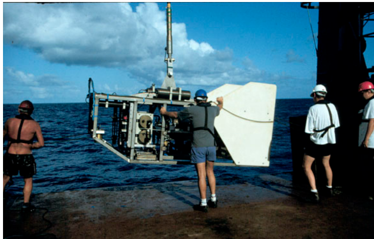
Figure 11: The Southampton Oceanography Centre's deep-tow hydrothermal plume instrument BRIDGET being prepared for launch from the RRS Charles Darwin at the Mid-Atlantic Ridge
