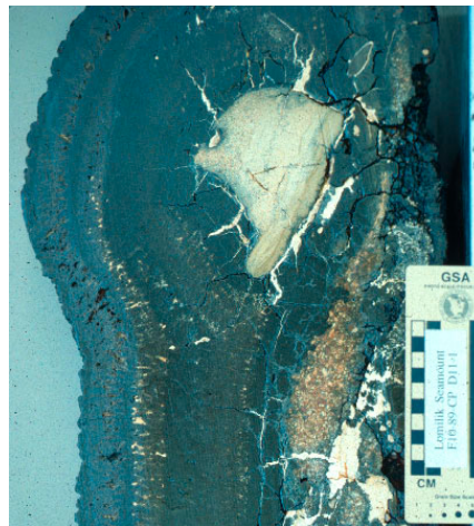
Appendix 1. A. Fe-Mn crust pavement (~3 x 4m) on the upper flank of Horizon Guyot, Central Pacific; 2000 m water depth. B. Large sample (1.5 x 0.9 x 0.3 m) of cobalt-rich Fe-Mn crust and substrate rock; typical botryoidal surface. C. Same sample as in (B) cut through the long axis. The Fe-Mn crust is about 18 cm thick and shows distinct growth layers. The crust grew on a volcaniclastic substrate rock and growth started 60 Ma ago. A mudstone cobble occurs within the crust on the right side.
