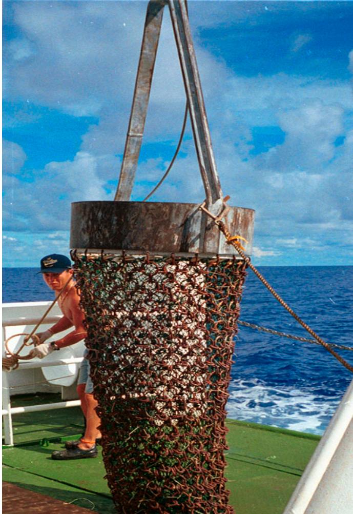
Appendix 4. 1-m-diameter circular chain-bag dredge used to sample seamounts.
