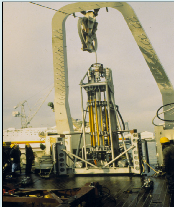
Figure 6: Australian PROD drill for coring tens of metres into the seafloor. The drill assembly is deployed from the ship to the seafloor. Final positioning is achieved by means of thrusters. A new core barrel is rotated into position as the preceding one is filled.
