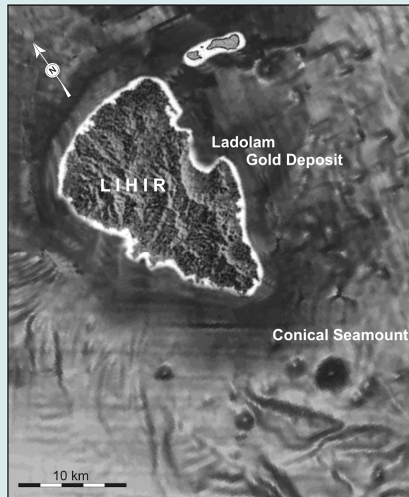
Figure 6: Bathymetry-based shaded relief of the Lihir Island group with the location of volcanic cones south of Lihir including Conical Seamount, which is host to a new type of submarine gold mineralization.
