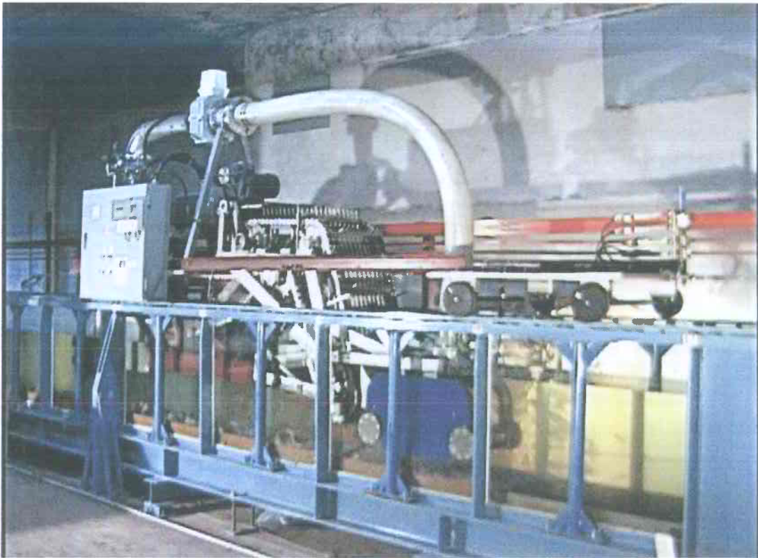
Figure 2 - Model Test of Hybrid Nodule Pick-Up Device at KRISO
