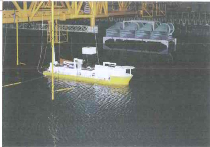
Figure 7 - DP Simulation of Drillship in Waves, Wind and Current and below, a Mining Ship Model Test
