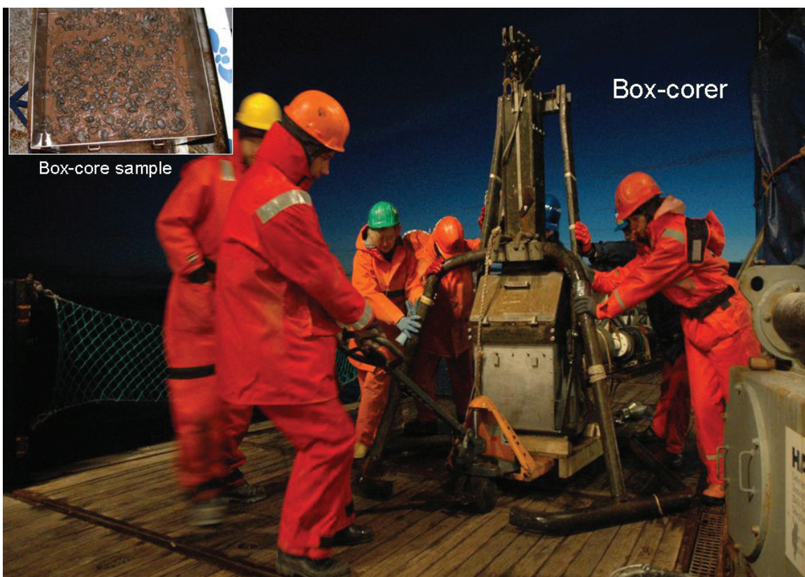
Figure 2. The USNEL type box corer in the process of sample box removal. Insert: Vertical view of the box core sample (0.25 m 2 in area), with manganese nodules on the sediment surface. Photos: P. Martinez and C. Smith (inset).
