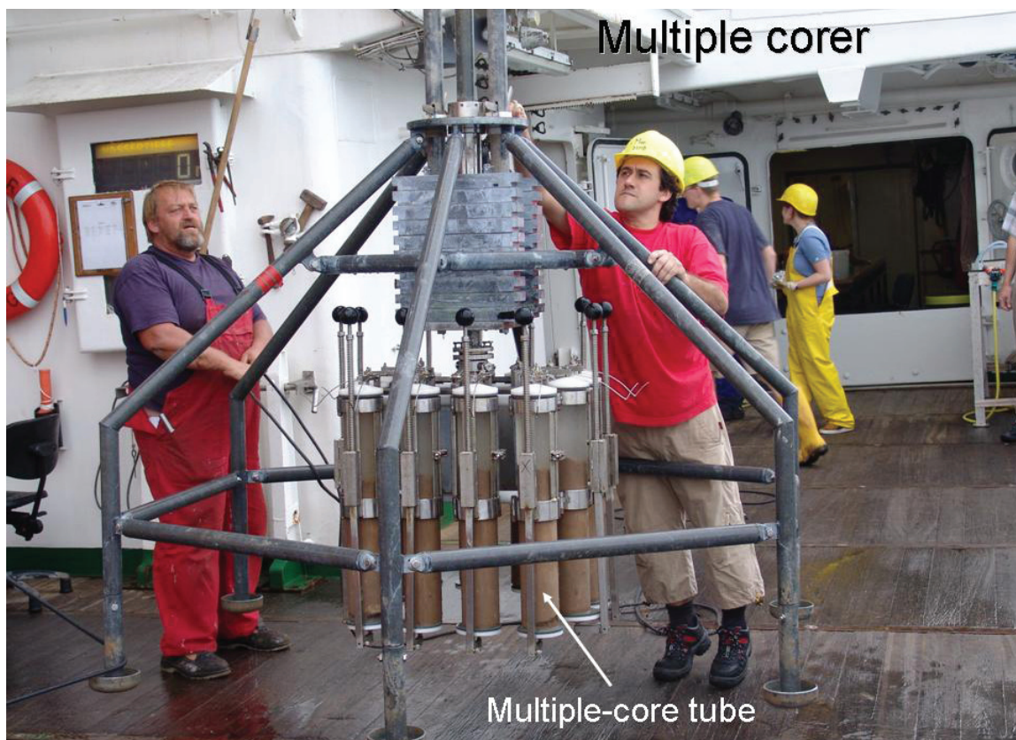
Figure 3. Multiple corer during recovery from sampling. The multiple corer collects 12 tube samples (each 80 cm 2 ) in area. Photo courtesy of P. Martinez.
