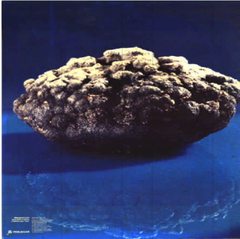
Figure 18. Photo of an individual polymetallic manganese nodule specimen (about the size of a golf ball)
