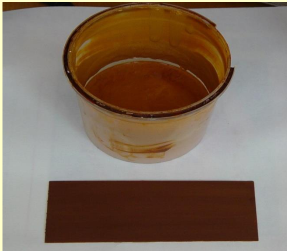
Antirust dope made from acid leaching residues and its pain-coat
