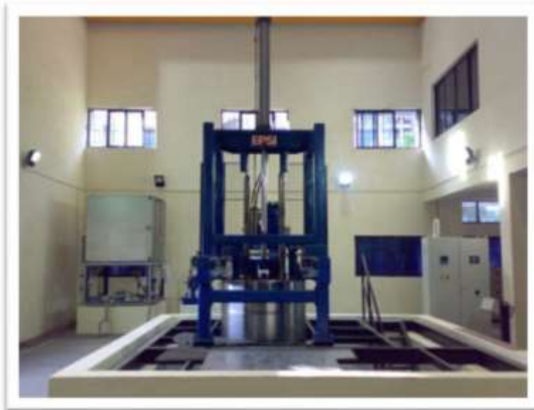
Figure 13: Hyperbaric chamber Test components can be placed inside the vessel and pressurized using a high pressure pump. A programmable logic controller is used to set parameters including set pressure and dwell time.
