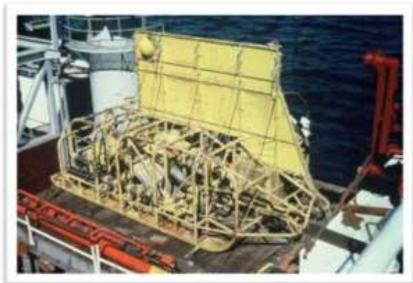
Figure 8: Two-metre DOMCO hydraulic collector
