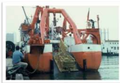
Figure 7: Dockside testing of collector launch and recovery procedures on the R/V Valdivia
