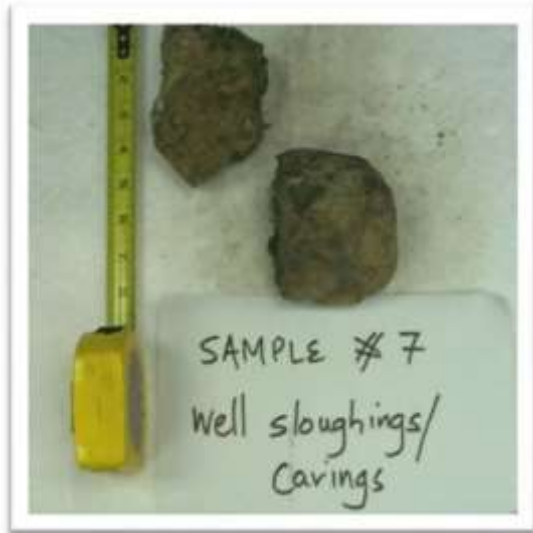
Figure 20: Solids pumped through the SMP
