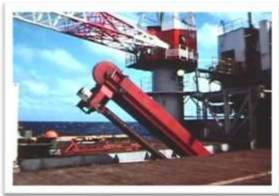
Figure 3: Pipe handling equipment aboard the SEDCO 445
