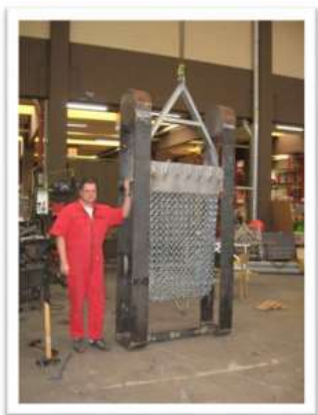
Figure 6: Chain-sack dredge adapted for use during the upcoming exploration cruise to the German licence area. The dredge has been fitted into a frame which is thought to prevent the sampling instrument from sinking into soft sediments and enabling sliding at the nodule-covered surface.
