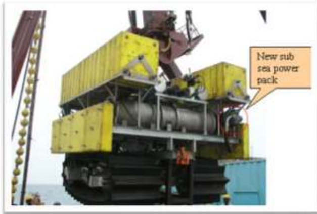
Figure 7: Underwater crawler with new sub-sea power pack being launched
