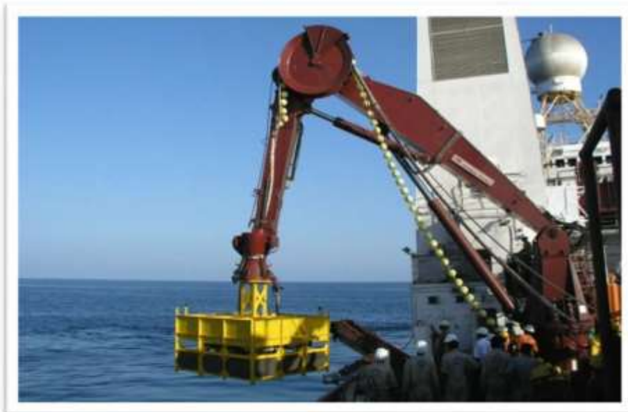
Figure 2: Launch and Retrieval System (LARS) and DP Systems being tested using a dummy load similar to the underwater mining machine
