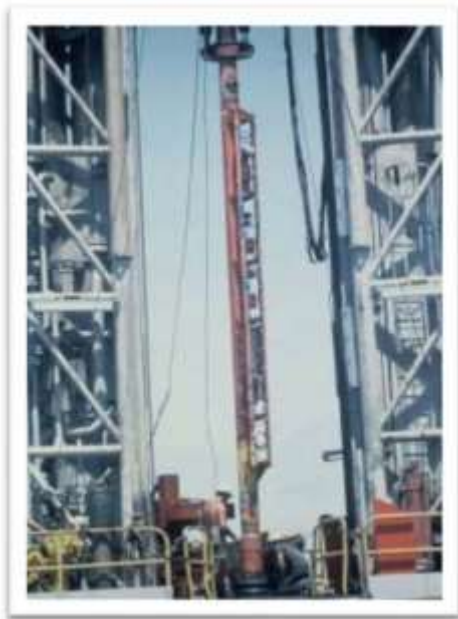
Figure 14: Instrumentation sub being integrated into the riser
