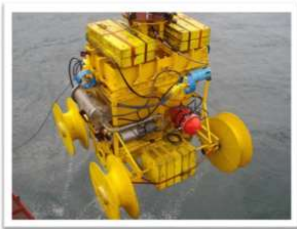
Figure 8: Artificial nodule laying system being launched
