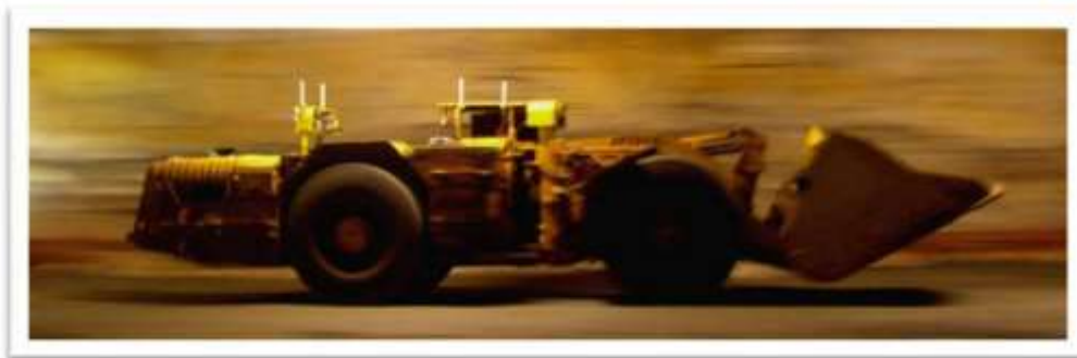
Figure 2: Underground LHD vehicle driving autonomously with no infrastructure
