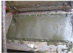
Smith-McIntyre Grab with full bite of sediment
