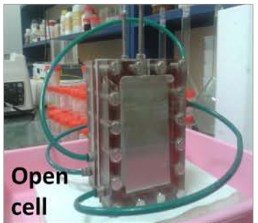
Open cell Development of salt splitting cell at lab scale of 6L/h capacity
