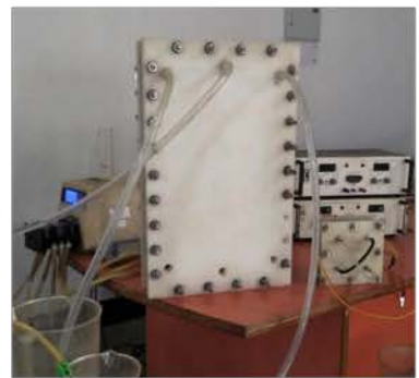
Up-scaled cell of 50L/h capacity
