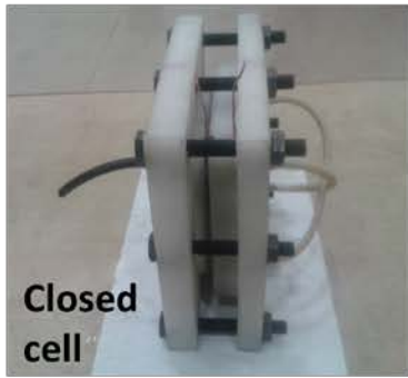
Open cell Development of salt splitting cell at lab scale of 6L/h capacity
