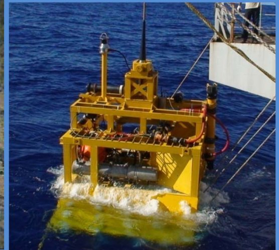
In-situ Soil tester in splash zone
