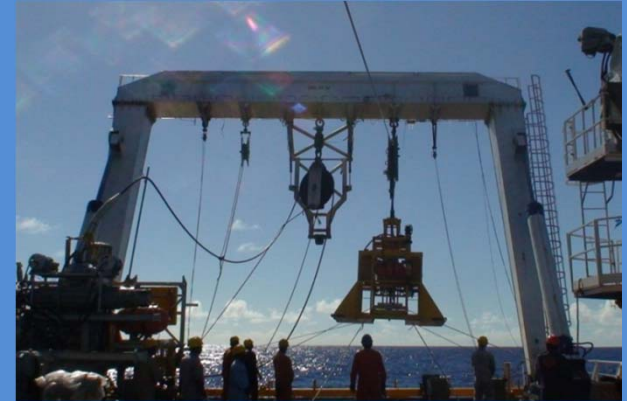
Launching of In-situ Soil tester
