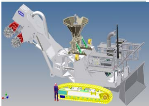
Auxiliary Cutter — cuts ore on uneven surfaces; benching the site
