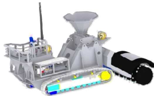
Bulk Cutter — cuts ore at high rates on areas benched by Auxiliary Cutter
