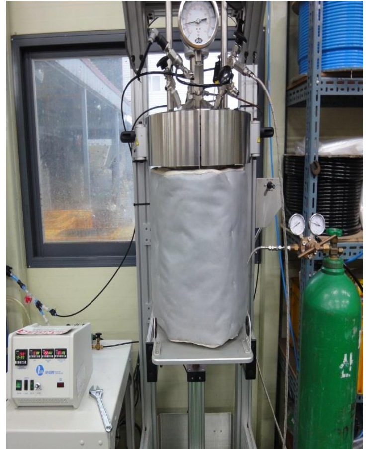
Batch type autoclave (15 Liter)
