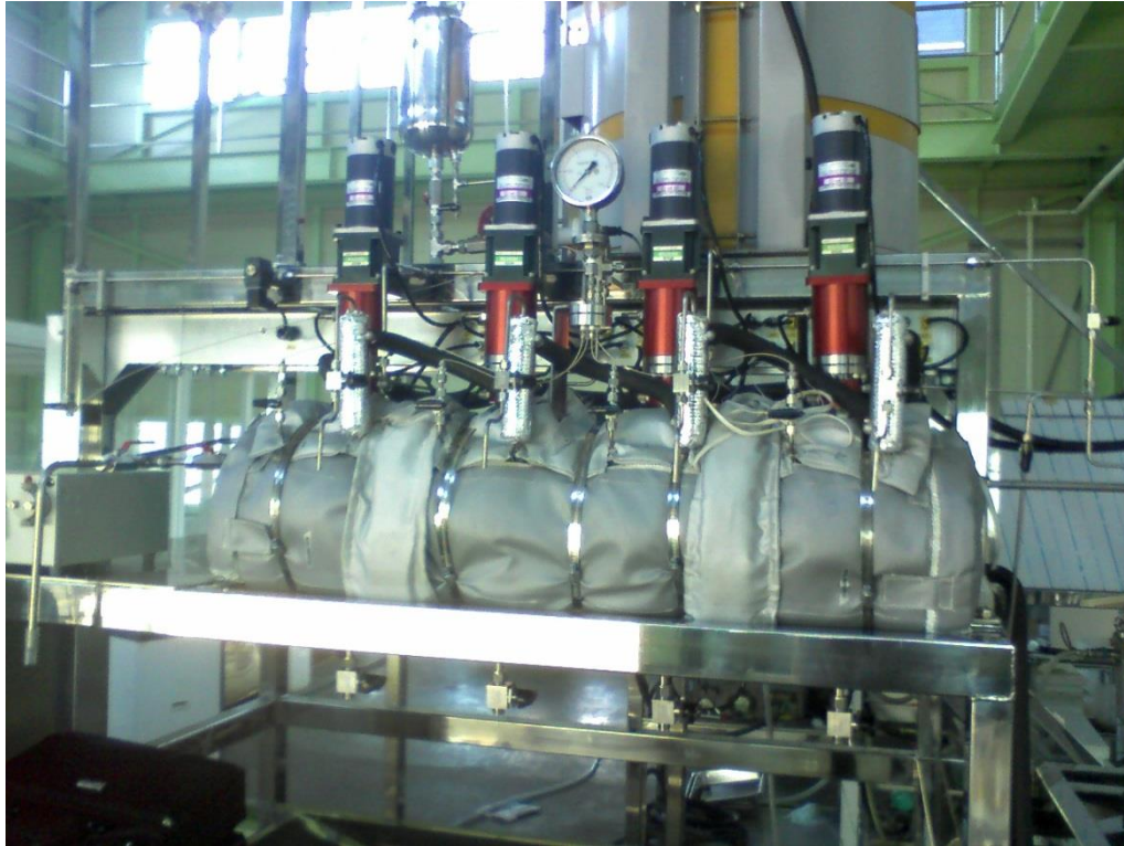
Continuous type autoclave (40 Liter)
