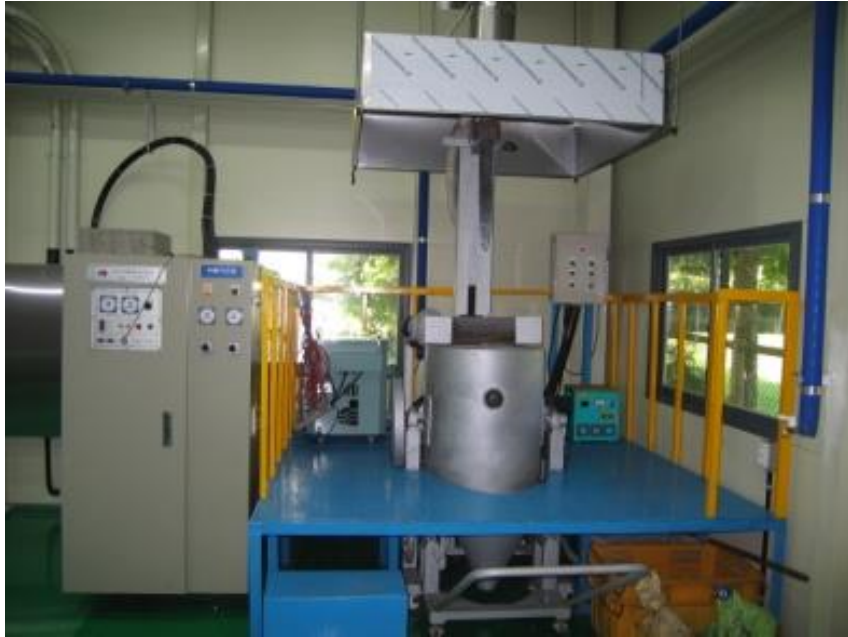
DC Arc Furnace (Batch type, 50kg/Ch.)
