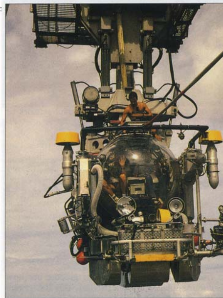
Figure 19.32 Some of the submersibles used for investigation of the deep ocean. (a) The French submersible, Cyana , capable of operating to depths of 4000 m. The hull is titanium, and the submersible carries a pilot, navigator, and one scientist. It is usually equipped with underwater lights, an arm, claw, and video. (Courtesy of Professor P. Tyler, SOC.) (b) The Russian Mir I submersible, capable of operating to 6000 m carrying two pilots and a scientist. The hull is titanium. The submersible is here carrying a (red) sediment trap, and still and video cameras; it has been used to investigate hydrothermal systems in the North Atlantic (see Chapter 13). (Courtesy of Professor P. Tyler, SOC.) (c) The US Johnson Sealink submersible in preparation for deployment. It is capable of operating to 900 m with a pilot and scientist in the front compartment and with a technician and second scientist in an aft compartment. The sphere is acrylic. In addition to lights and cameras, the submersible has a manipulation claw. (Courtesy of Professor P. Tyler, SOC.) (d) The US Navy-owned Deep Submergence Vehicle (DSV) Alvin operated by the Woods Hole Oceanographic Institution. A typical 8 hr dive takes two scientists and pilot to 4500 m with 4 hours on the bottom for observation, photography, and experiments. Three video and two 800 frame cameras are usually carried, together with two hydraulic arms and instruments such as corers, temperature probes, water samplers, and a biological sample pump. (Courtesy of Woods Hole Oceanographic Institution.)
