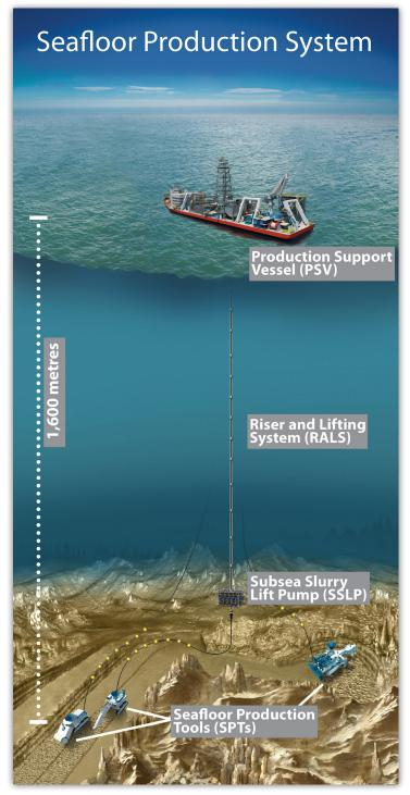
An example of a commercial seabed mining system. @ Nautilus minerals
