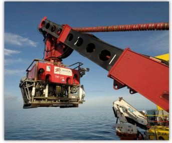
A remotely operated vehicle ROV) being deployed to study the seafloor. © Nautilus Minerals
