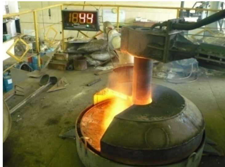
DC arc Furnace smelting Mn Nodules
