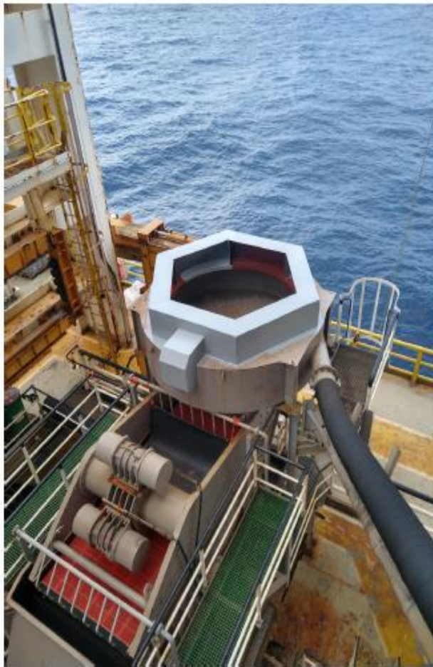
Figure 6 : Modifications to the cyclone feeder – increased height and overflow bypass onto the separator deck.
