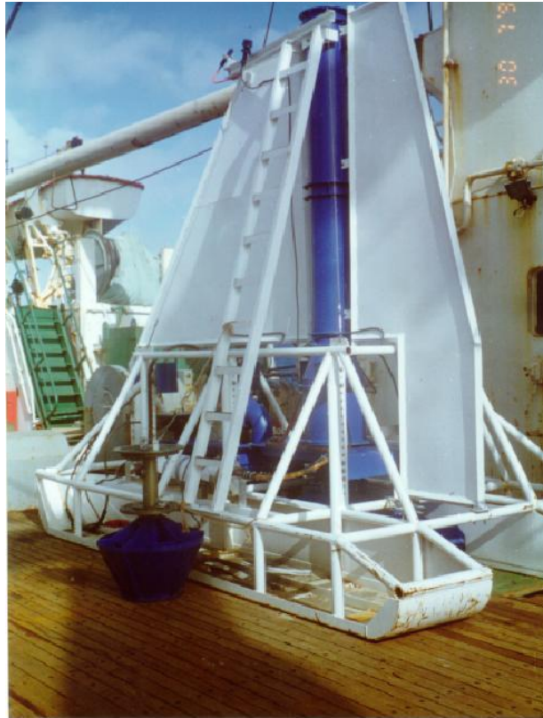
Fig.6.2.5.3.1: Deep-sea sediment resuspension system
