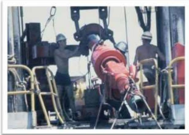
*Figure 10: Dump valve being lifted to rig floor*
