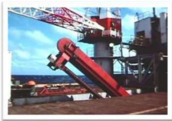
*Figure 3: Pipe handling equipment aboard the SEDCO 445*
