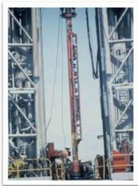
*Figure 14: Instrumentation sub being integrated into the riser*
