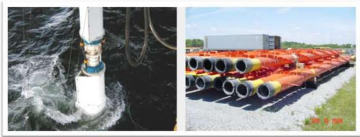
The strakes may be preinstalled on the risers and the risers may be stacked closely together.
