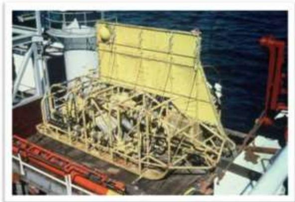
*Figure 8: Two-metre DOMCO hydraulic collector*
