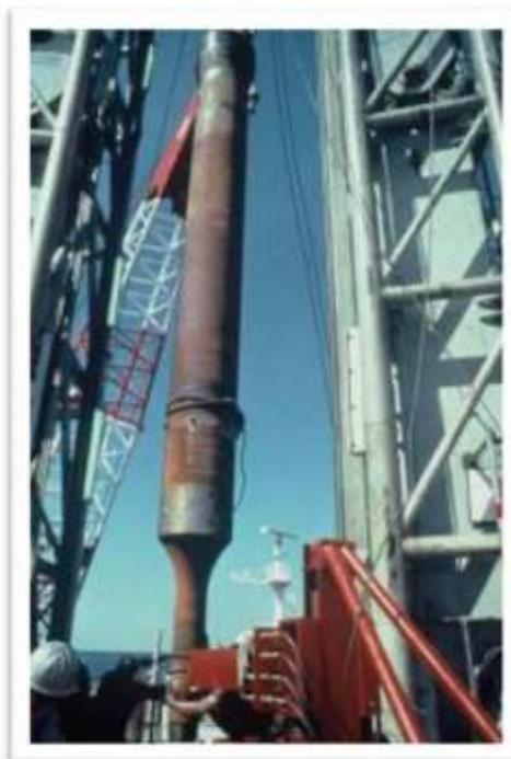
*Figure 12: In-line submersible pump*
