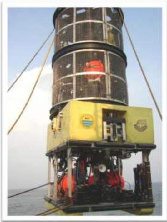
*Figure 14: ROV being launched*
