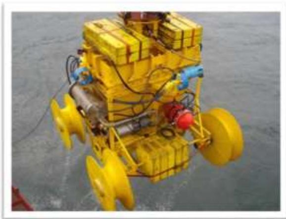
*Figure 8: Artificial nodule laying system being launched*
