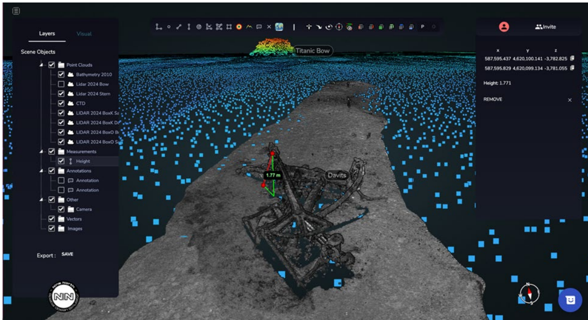
Figure 2: DeepMap, displaying a high-resolution Lidar made in 2024 on the bathymetry from 2010.
